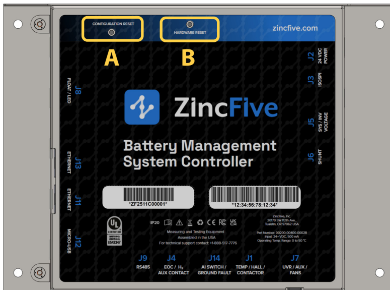
Figure 15- ZincFive BMS Controller buttons A- Configuration Reset button, B- Configuration Reset button
