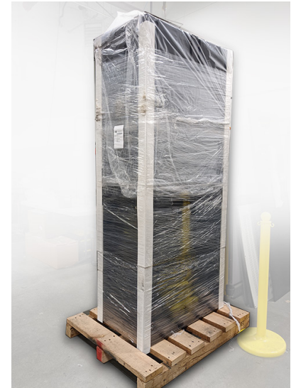
Figure 2. Palletized Battery Cabinet Packaging.
